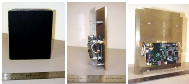
Fig. 2. UWB Perimeter Intrusion Detection Sensor Hardware.
