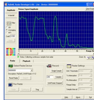
Figure 10. RADEKL Graphical User Interface (GUI) (Return through multiple walls in office building)
