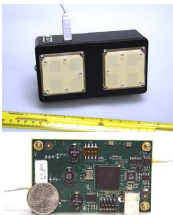
Figure 8. RADEKL UWB Radar Sensor with Single Board Design (antenna radome removed)
