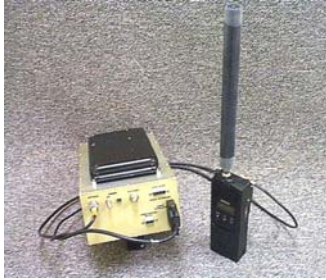
Figure 2. Draco UWB Communications Node MBITR handheld interface on right, UWB transceiver with NPU unit on left.
