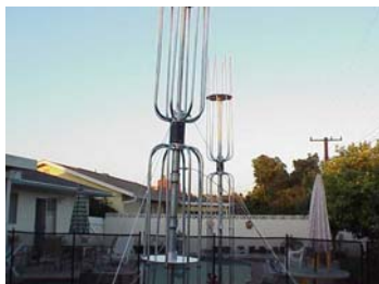
Figure 6. HFUWB "Fat Dipole" for 30-50 MHz Coverage
