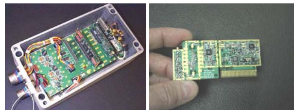
Figure 4. Modular HFUWB UWB Transceiver (Transceiver shown with RF front end module)
