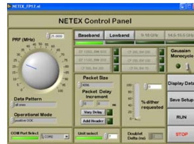
Figure 12. LabVIEW Interface for UWB Generator
