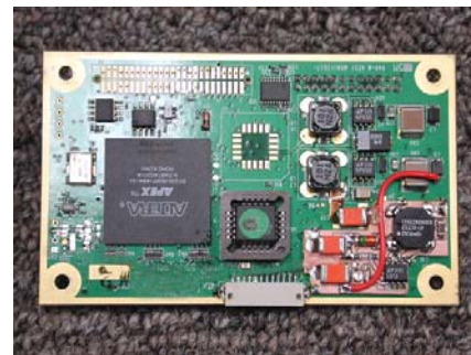
(a) Front – CVSD Codec, Controller & Power Supplies
