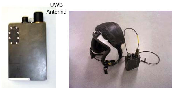
Figure 8. Prototype AWICS UWB Mobile Transceiver with Headset
