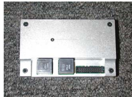
Figure 4. AWICS UWB Transceiver Module (3 5 / 8 x 2 3 / 8 x 1 inches)
