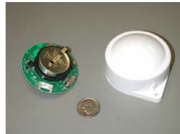
Figure 1. PAL650 UWB Active Tag with Radome
